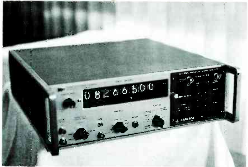
FIG. 1—THE PANEL-MOUNTED VERSION of the prescaler, in an HP 5245L frequency counter. The HP5245L is often available as surplus for about $200, and the prescaler is a good way to update it.
