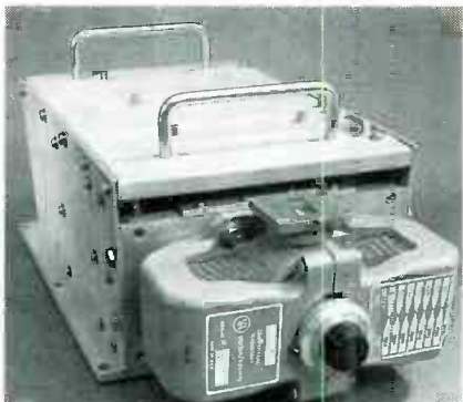
FIG. 9—THE VARIAN SFD-352 TUNABLE, conventional magnetron; the output waveguide flange appears on the top of the front. It has a tuning range of 8.5–9.6 GHz set by the vernier, a peak power of 220 kilowatts, a nominal anode potential of 22 kilovolts, and a peak anode current of 28 amps.
